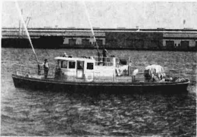
Testing water monitors on prototype of model fireboat at Long Beach, California. Water monitors on model are remote controlled.
