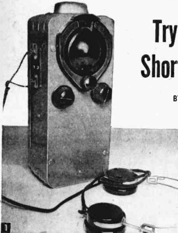
Portable receiver brings in short-wave signals from a surprising distance. Vernier tuning dial helps to separate stations.
