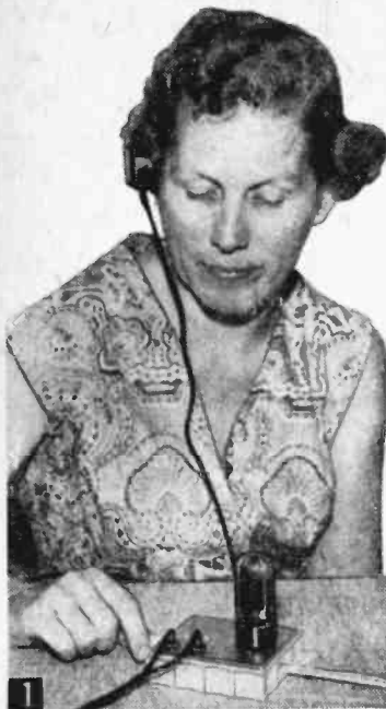
1 Mounted in a plastic jewelry box, this powerful one-tube all-electric radio sets a record for compactness. The .117L M7 tube serves as both screen-grid detector and rectifier.
