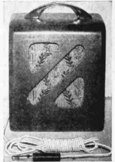
2 Intercom or dressed-up cigar box houses 4 or 5-in. speaker. Extension cord is ordinary fixture wire.
