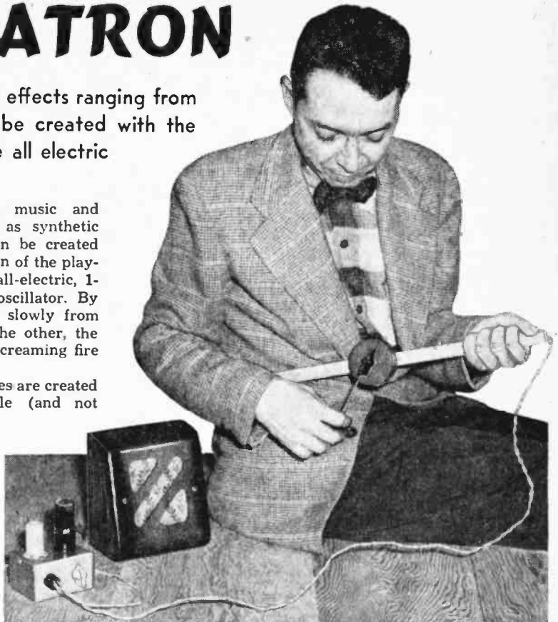
1 The Uke-Atron, an electronic playing device, is held guitar fashion. PM speaker, mounted in standard wooden cabinet, and oscillator unit appear in foreground of photo.
