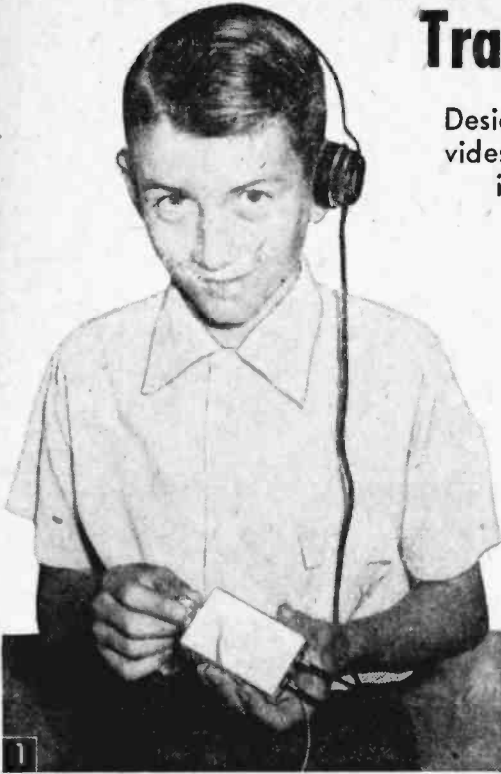
Pocket transistor radio for headphone listening operates most anywhere, usually without outside antenna. Single alnico 1000-ohm phone provides good volume. Double headphones up to 4000 ohms will provide more volume if desired.
