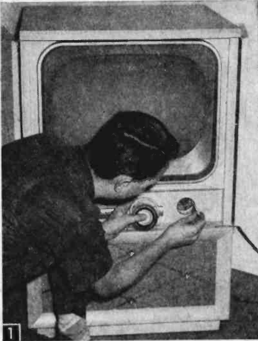
Fig. 1. Occasionally, adjustment of tuner oscillator coil slugs will restore picture sharpness. To reach slugs, pull off station and fine tuning knobs. Fig. 1A. Coil boards on turret tuners may be snapped out of drum for replacing with a UHF channel. Clean silver buttons with Carbona occasionally to remove leakage paths caused by dust and minute metal particles.
