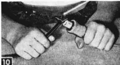
Shank of a hot soldering iron drawn between wires of oval lead-in wire will melt and seal the air core against moisture (see text).
