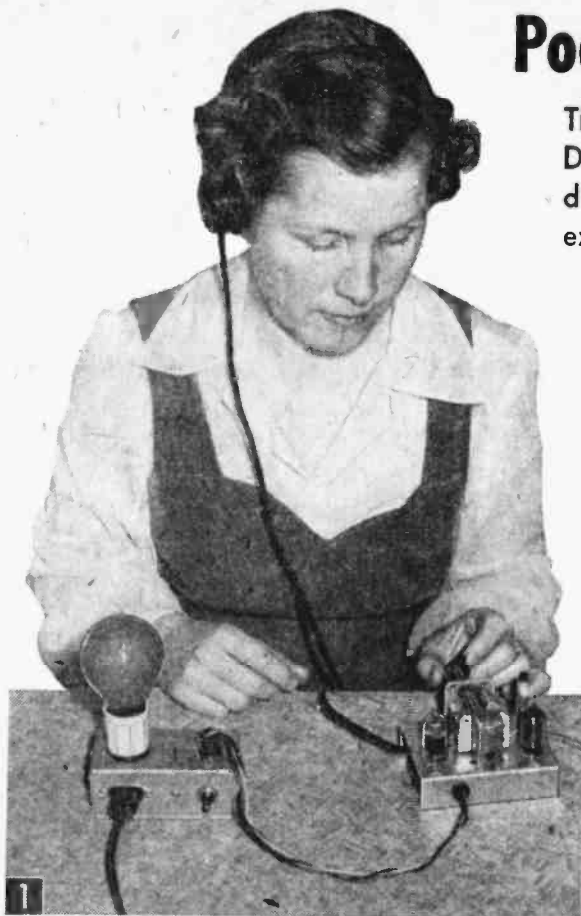
1 Pocket-size power pack supplies d-c and heater voltages to midjet superhet tuner. Power Pack operates all types of electronic apparatus where d-c current is not over 100 ma.
