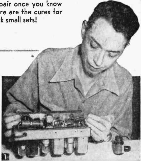
DIFFICULT TUNING. Slipping dial cord produces backlash. Apply mixture of 1 drop thick bone glue mixed with 1 drop glycerin to cord shaft of dial drive (See 1, Fig. 3). Or take up slack in dial cord caused by wear.
